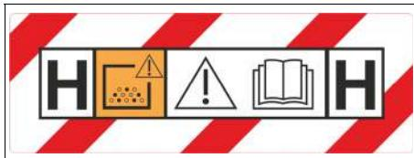
**WARNING:** This machine contains dust that is harmful to your health. Emptying and maintenance, including removal of the dust bag, may only be performed by technical specialists wearing suitable personal protective equipment. Do not operate the device without the complete filtration system.
