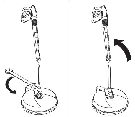
→ Connect the steel pipe of the high pressure cleaner to the FR Basic and tighten it with wrenches (width 24).
