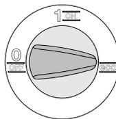
There are the switch positions "1/ON" and "eco" to switch the appliance on.
